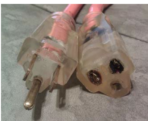
Extension cord electrical arc damage
